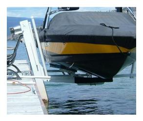
With concern of rough water conditions, have the lift bed slightly higher for leaving the lift under more power in reverse gear.
